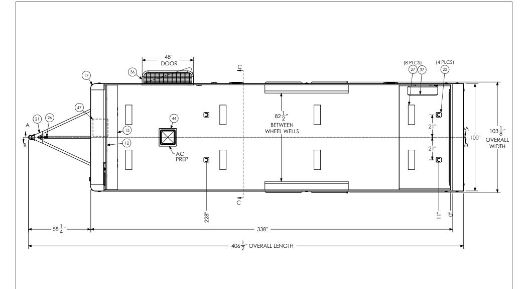
inTech Trailers SCALE: 1:45 NAME DATE inTech 2/7/24 DRAWN ALL DIMENSIONS ARE IN INCHES AND ARE NOMINAL. DIMENSIONS ON ACTUAL TRAILER MAY VARY FROM WHAT IS SHOWN ON PRINT BASED ON ACTUAL FRAMING AND TRAILER STRUCTURE, UNLESS NOTED AS CRITICAL BTL8.5x28TA3 - STANDARD **FLOORPLAN**
